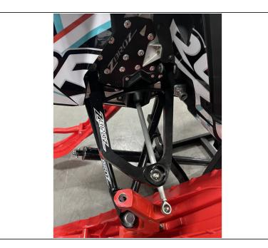
IMAGE 3 Next Install the new uppers into the pivot location making sure to reuse the stock washers in the correct location. Also be careful to insure the rear mounting nut doesn't fall back into the engine bay. Leave the ball undone until you have the shock installed.
